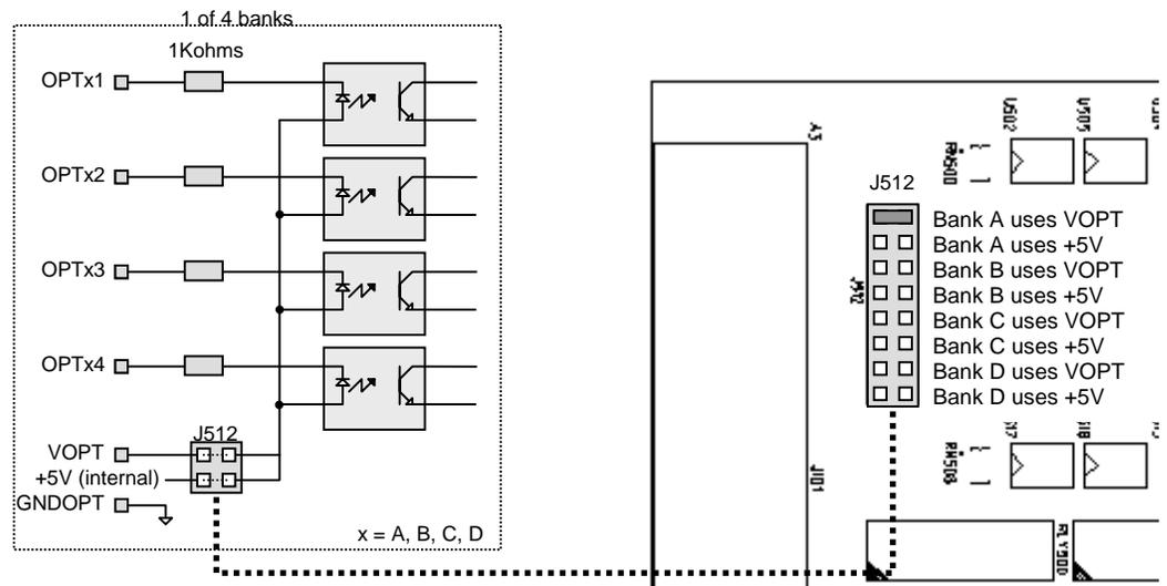
The following diagram shows the connections needed if using the internal +5V to power the opto-isolators.
