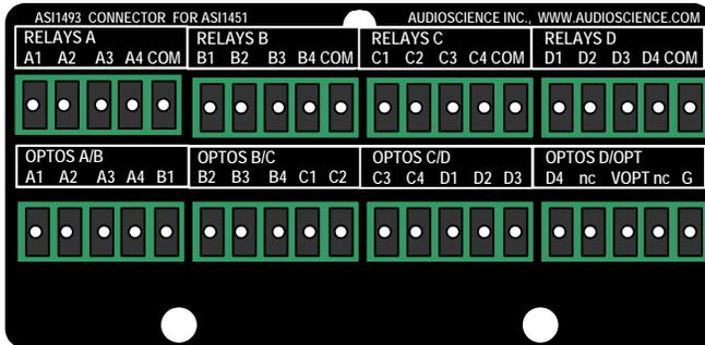
The ASI1493 Terminal Block Module connector provides a 3.81mm Phoenix type connector breakout option for the ASI1451.
