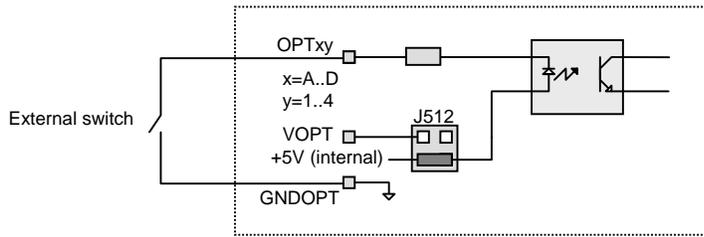
When using an external power source for the opto-isolators, use the following diagram as a guide to connections:
