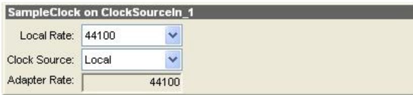
Figure 6. Clock Source information as seen in ASIControl.
