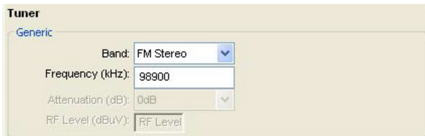
Figure 2. Generic section of Tuner controls.
