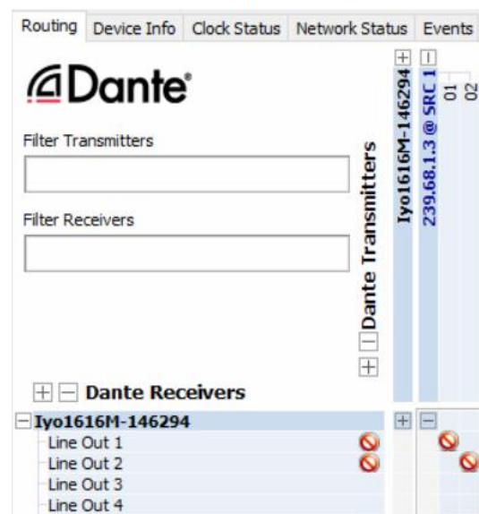
Figure 11 Dante Controller connection error
