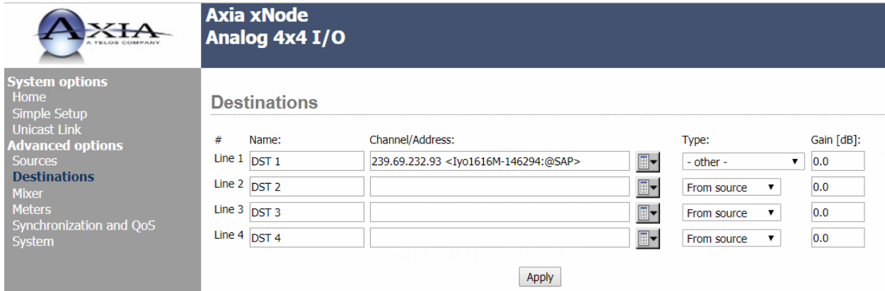
Figure 10 Connect Iyo Dante stereo Source to xNode Destination
