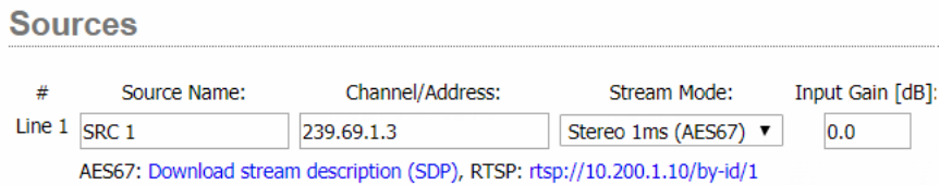
Figure 4 Axia xNode AES67 stereo source
